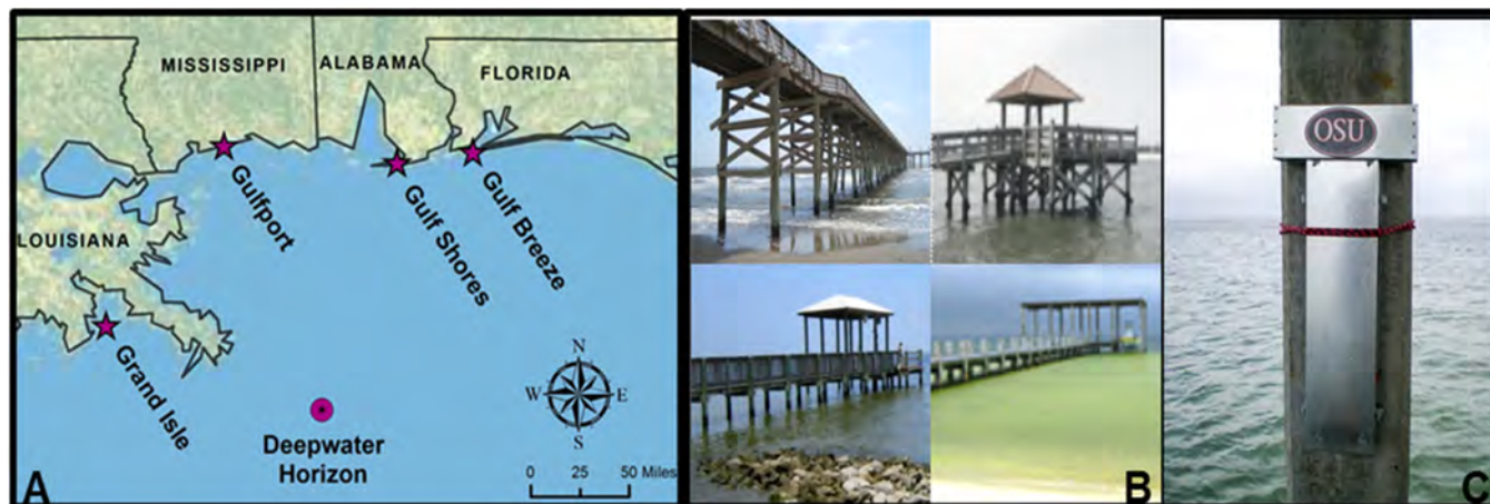
Figure 1. (A) Sampling locations along the Gulf of Mexico. (B) Samplers deployed off piers at each sampling site. (C) Air sampling cage affixed to pier in Gulf Breeze, FL.
