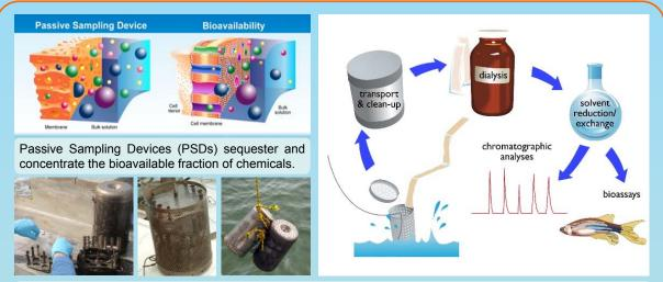
Sampling and Chemical Analysis: Low-density polyethylene tubing PSDs, were spiked with performance reference compounds (PRCs) and deployed in the water column. PSDs were extracted and analyzed by GC-MS for 33 PAH compounds. Water concentrations were calculated based on PRC diffusion rates<sup>(5)</sup>
