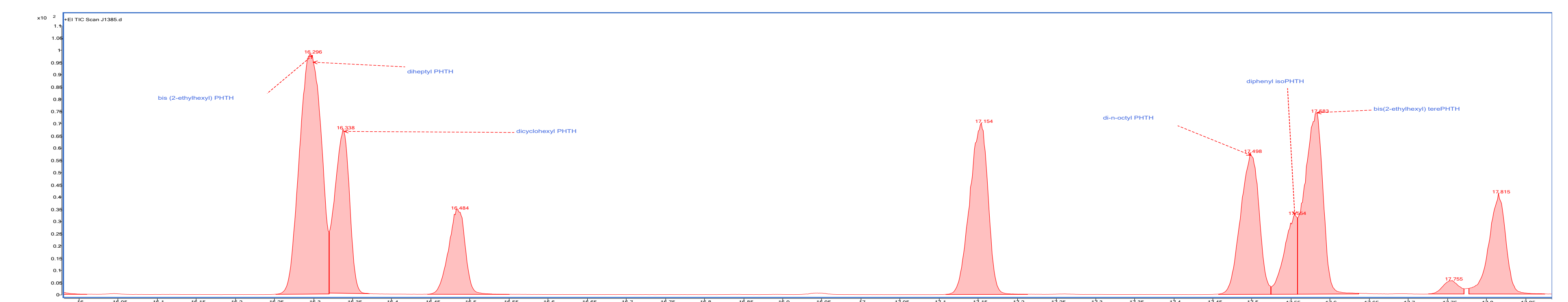
Figure 2: Coelutions in the method: bis (2-ethylhexyl) phthalate and diheptyl phthalate, diphenyl isophthalate and bis (2-ethylhexyl) terephthalate.
