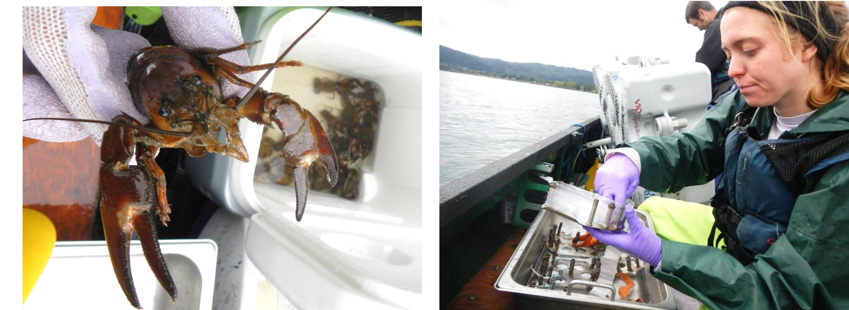
Figure 3. Signal crayfish, Pacifastacus leniusculus (left). Deploying LDPE passive sampling devices in Portland Harbor Superfund site (right).
