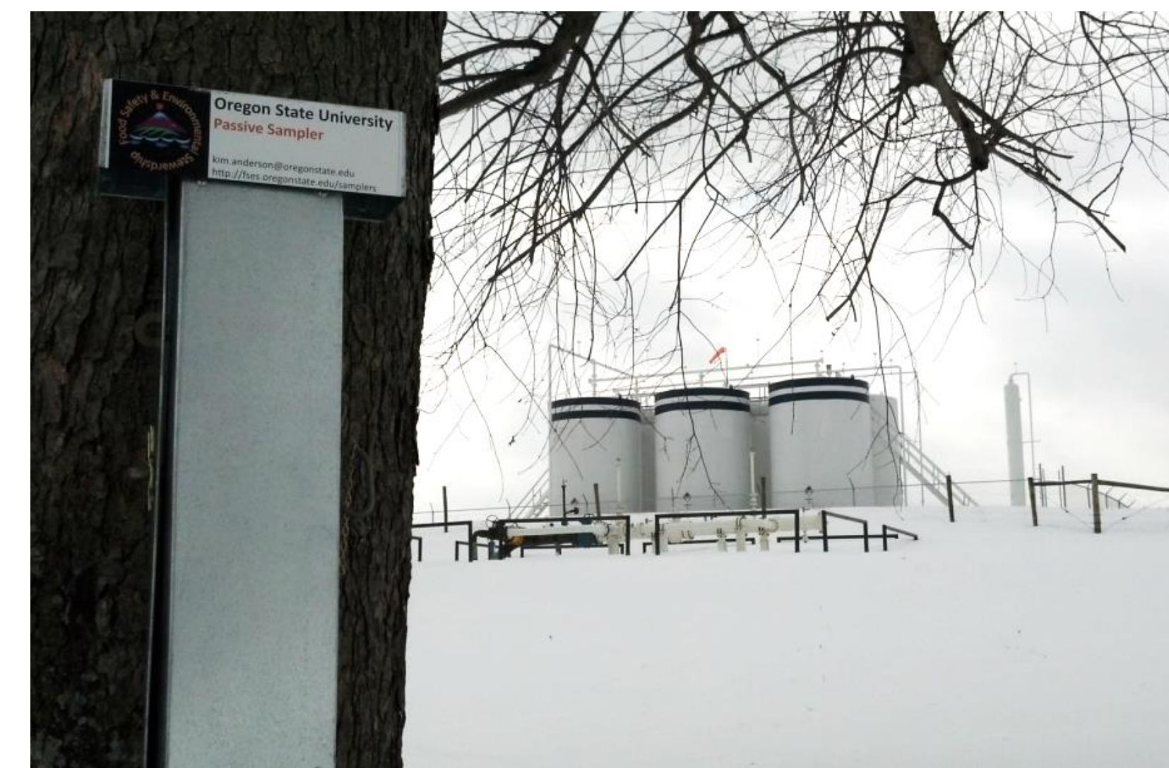
Air sampling cage with a producing fracking well pad in the background.
