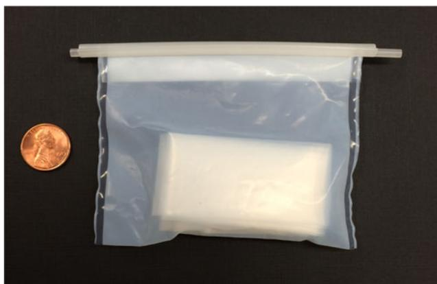
**Fig. 1** LDPE passive sampling strip in PTFE bag
